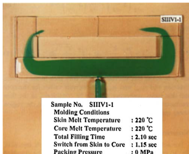
Figure 9. Sequential injection molded plate (cavity II) showing strong edge and corner effects.
